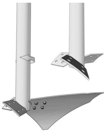
Axial flow helicoidal profile. Rotation direction: Clockwise, Thrust direction: downward Standard Bend
