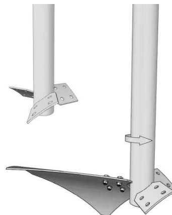
Axial flow helicoidal profile. Rotation direction: anti-Clockwise, Thrust direction: upward No-standard Bend
