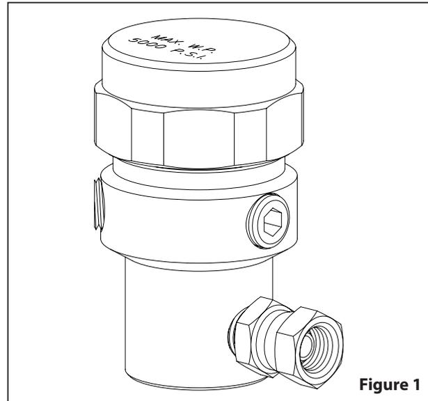
**WARNING** DISASSEMBLY HAZARD. Do not disassemble the filter when it is under pressure. Relieve pressure in the pumping system before attempting service or disassembly procedures. Disconnect air lines and carefully bleed pressure off the system. Be certain the system is not maintaining pressure due to a material restriction in the hose, line, dispensing device, or the spray or extrusion tip. Failure to relieve pressure, both upstream and downstream, may result in an injury upon disassembly.
